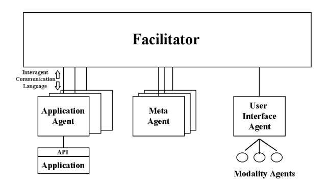
Figure 1: OAA System Structure.
